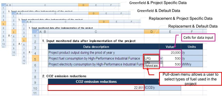
An example above provides different cases for greenfield project and existing (replacement) project and required data for each case.
