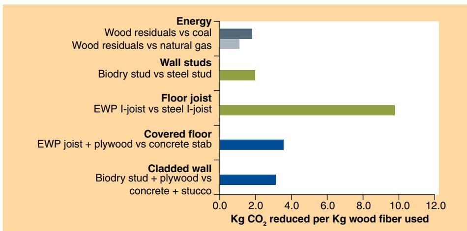
Figure 5. Carbon emission reduction by displacing non-wood products.
